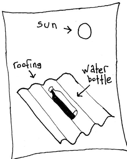
Figure 2-6: (Right) solar Distillation
