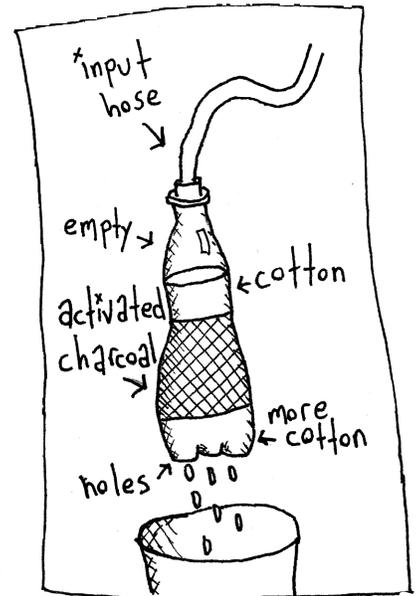
Figure 2-4: the Construction of a simple water Filter
